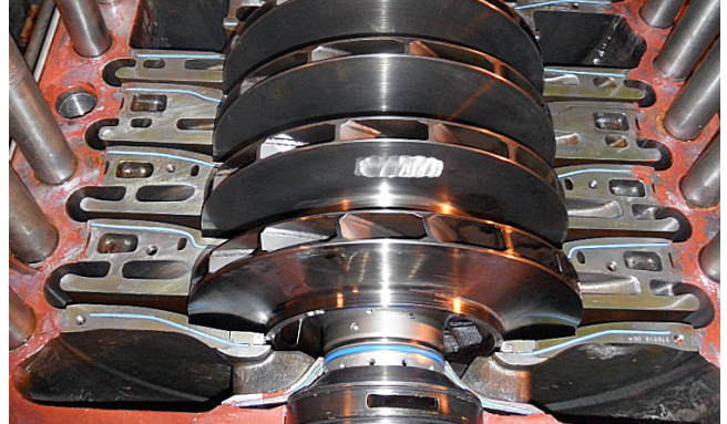
Non-Elliott compressor prior to rerate of flow path components.
