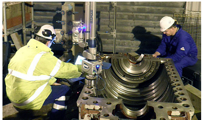
CMM inspection of casing bore in preparation for field machining new diaphragms.
